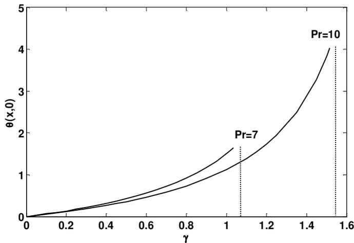
Figure 7: Variation of the wall temperature  $\theta(x,0)$  with conjugate parameter  $\gamma$  when  $Pr = 7$  and  $10$
