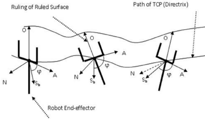
Figure 1: Ruled surface generated by  $O$  of tool frame
